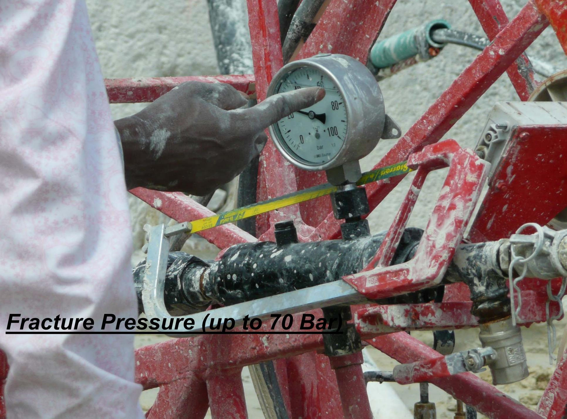
**Fracture Pressure (up to 70 Bar)**
