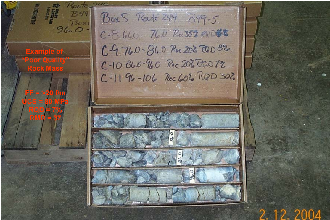
Figure 7. Example of "Poor Quality" Rock Mass
