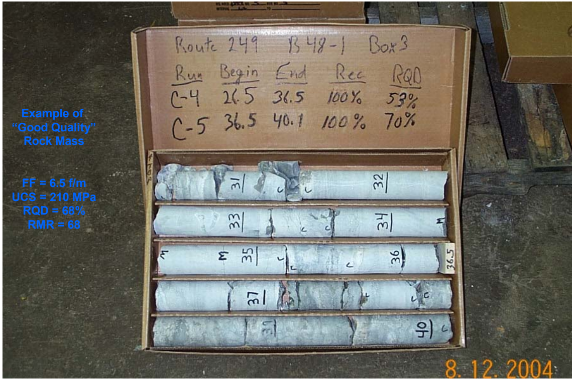
Figure 5. Example of “Good Quality” Rock Mass
