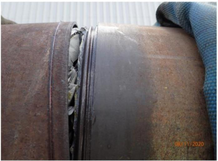
Predominant Failure Mode - Critical Cross-Section Failure
