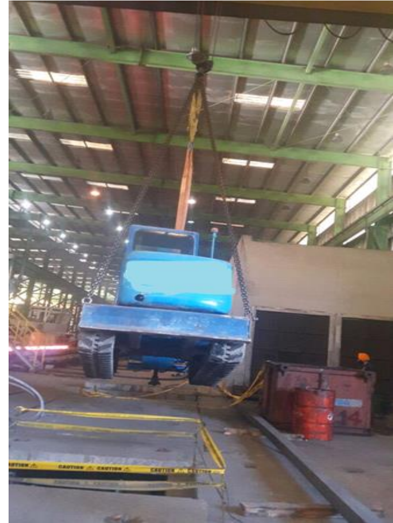
Figure 35: drill rig hanging on the overhead crane
