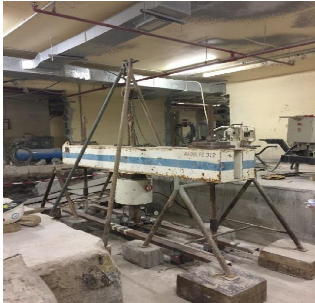
Figure 19: Pile testing set up
