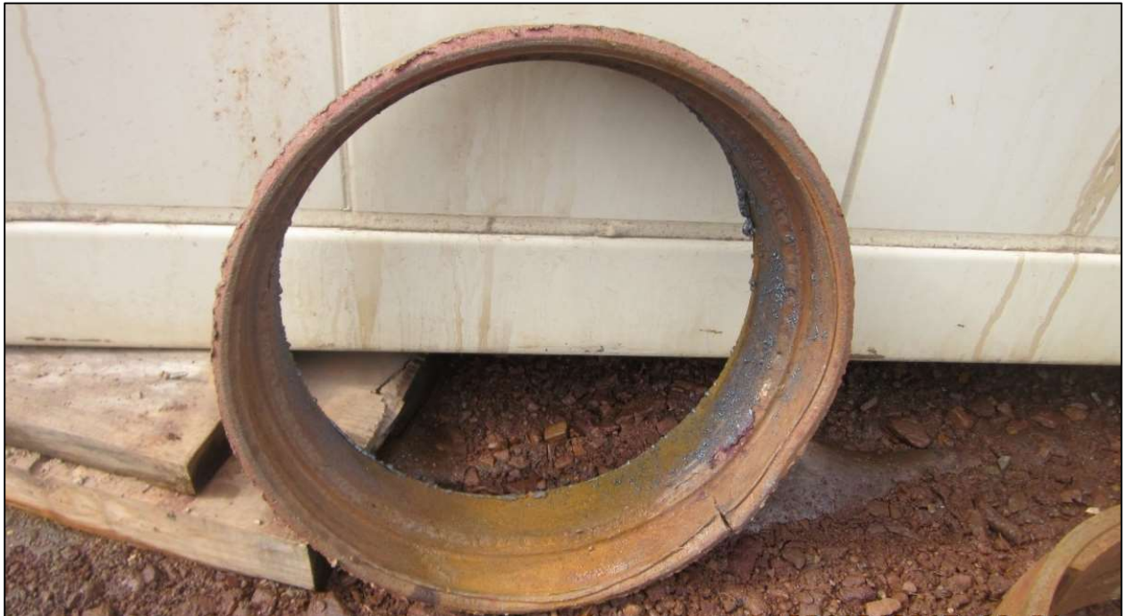
Figure 8: Damaged Elemex ring collar upon removal from casing.
