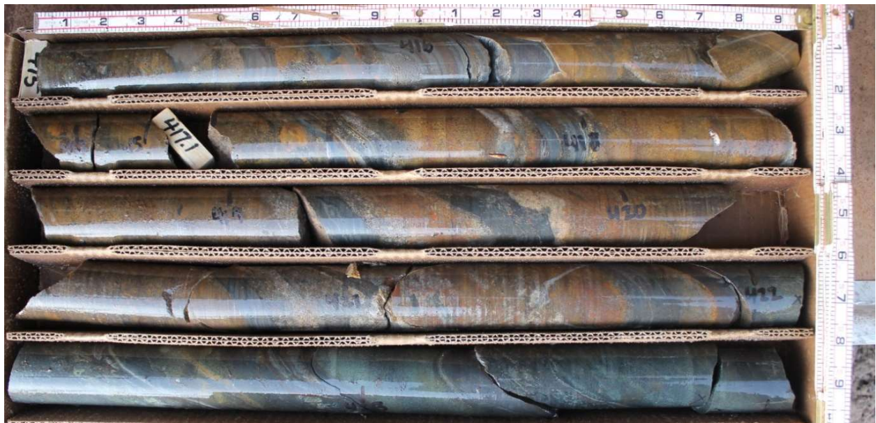
Figure 5: Biwabik Iron Formation rock core near the tip of the test pile.
