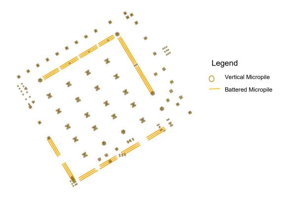
Figure 1. Initial pile layout with many lightly loaded piles.
