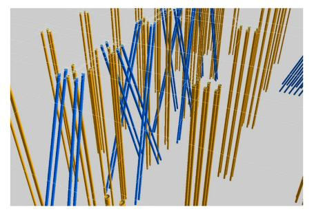
Figure 4. Revised battered and vertical shear key minimizing conflicts.
