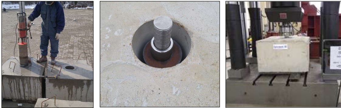
(a) RC footing coring (b) Ring plates attached to thread bar (c) Test set-up Figure 4. Preparation of specimens and test set-up
