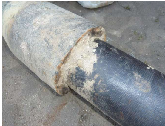
Figure 1 – coupling of DIP after 30 years
