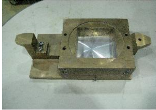
Figure 4. Picture of Aluminum in the lower part of direct shear box
