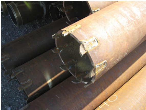
Figure 10. Initial Lead Casing Set-Up.
