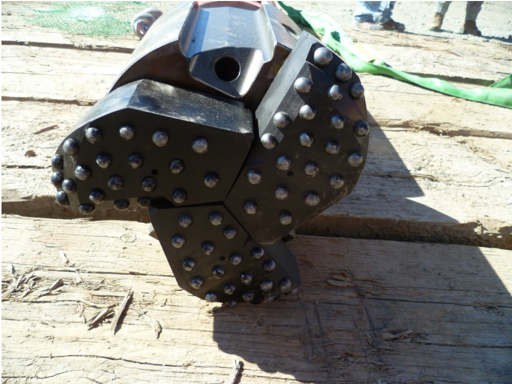
Figure 14. Down-The-Hole Hammer and Underreamer
