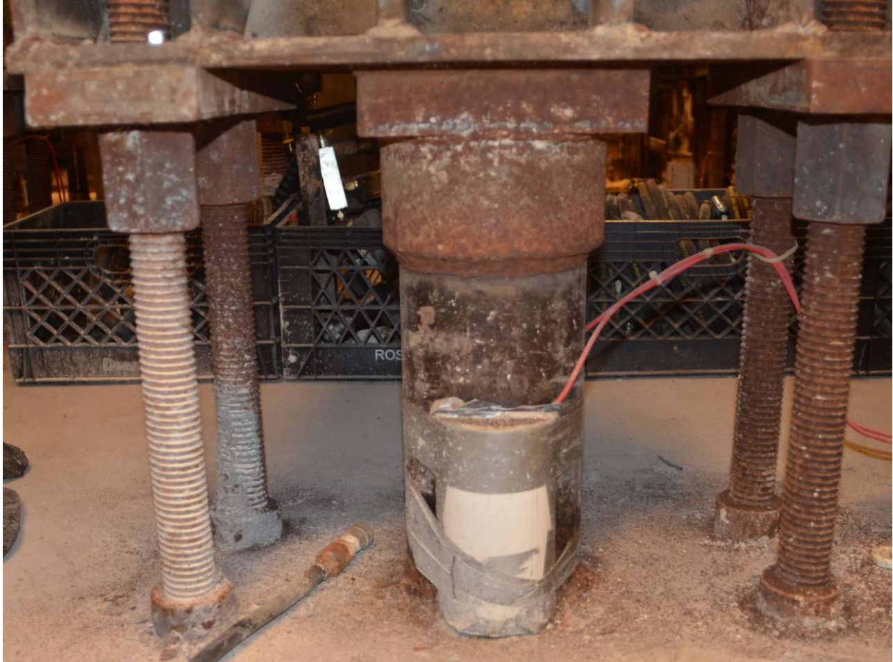
Figure 10 - VWSG's on Micropile L33 with PVC covers.
