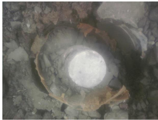
Figure 7 and 8. Pier 3 (left) and End Abutment (right) test micropiles after failure.
