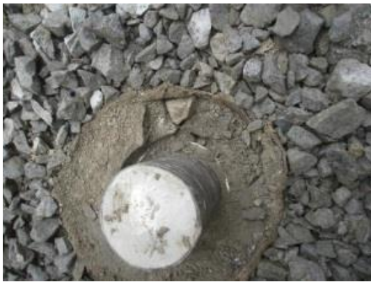
Figure 7 and 8. Pier 3 (left) and End Abutment (right) test micropiles after failure.
