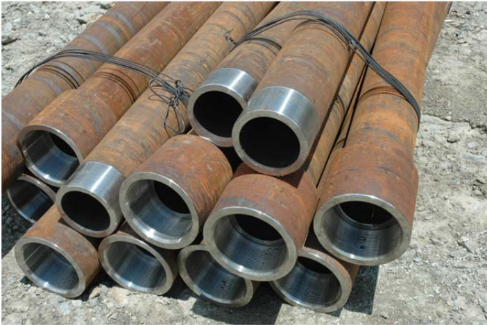
Figure 11. Casing used as micropile reinforcement.
