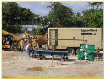
Figure 10: Micropile Tension Testing
