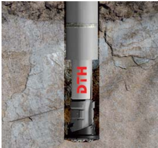
Figure 13. Continuing drilling with the pilot and the ring bit.
