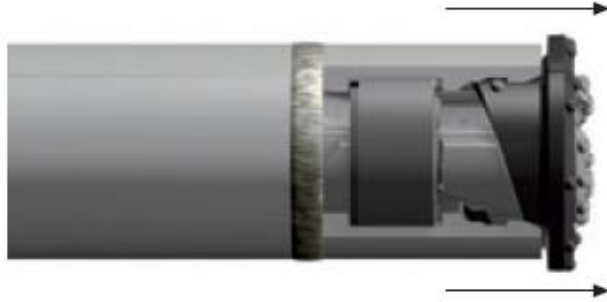
Figure 12. Feeding the drill string forward to slide the pilot through the drive ring.
