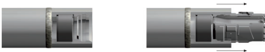
Figure 6. Driving the pilot through the casing and the casing extension.
