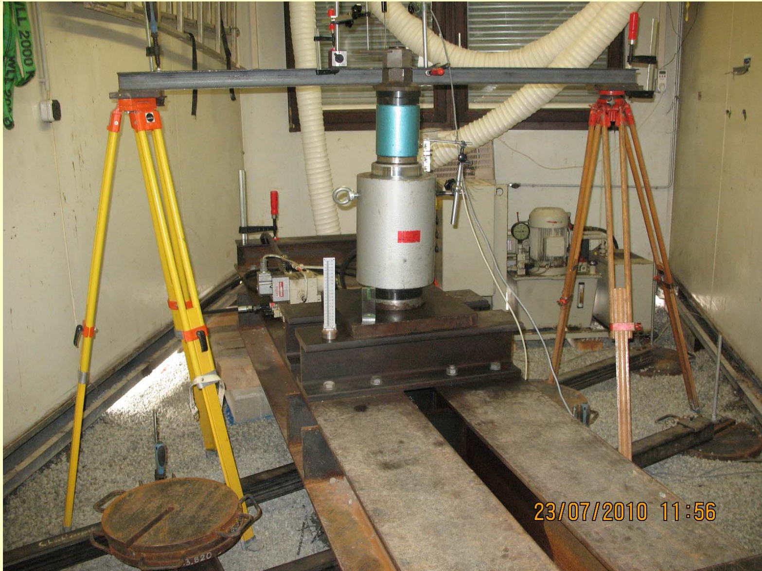
Testing set-up with load and datum beams
