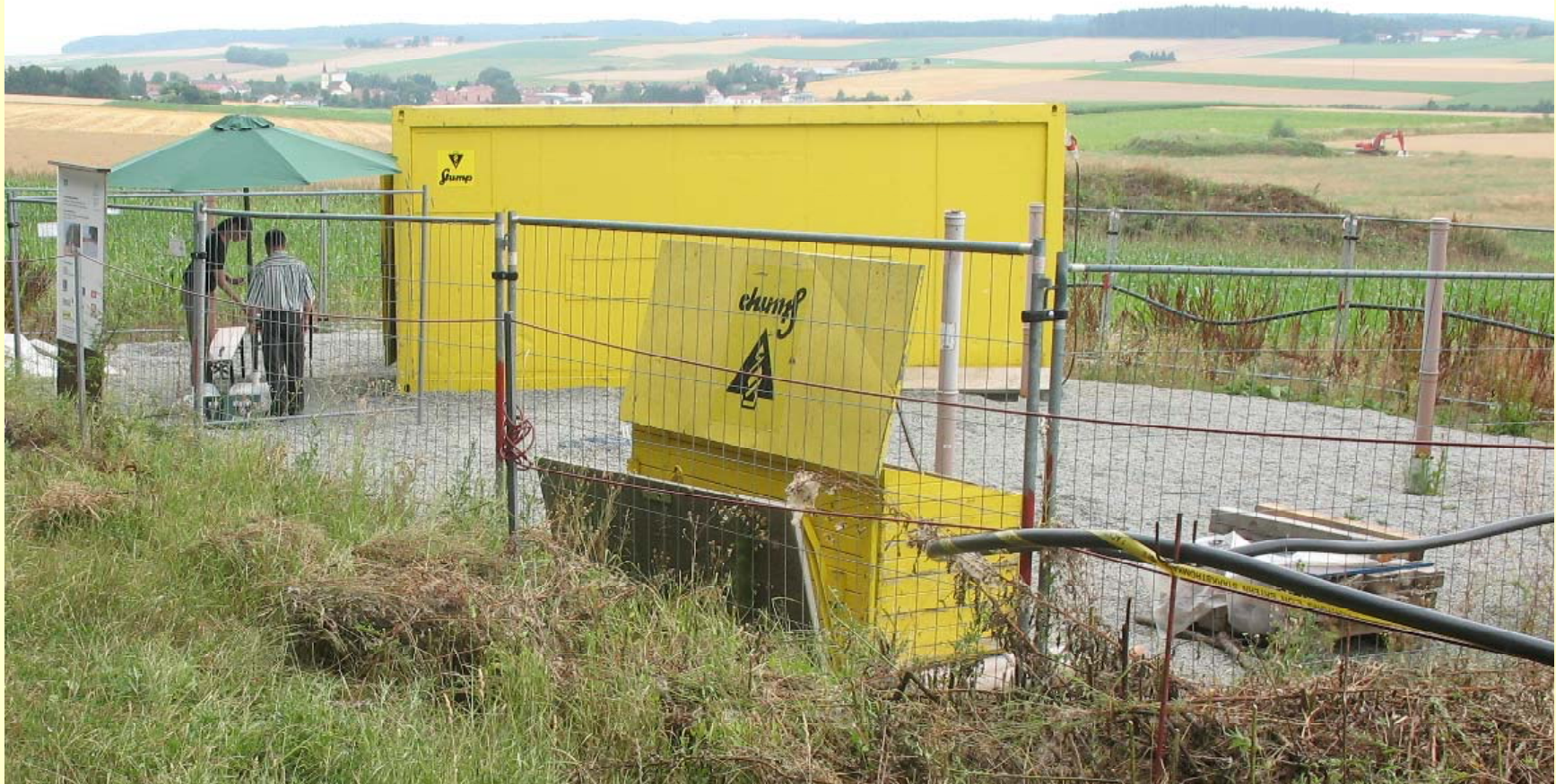
Test field with measuring container lifted onto each test pile
