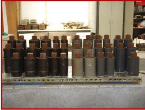
Confinement and micropile inserts
