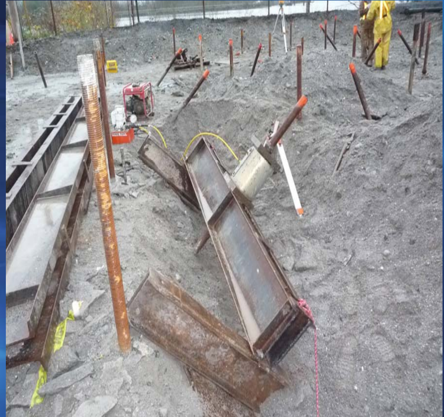
Tension Test Setup On Inclined Pile
