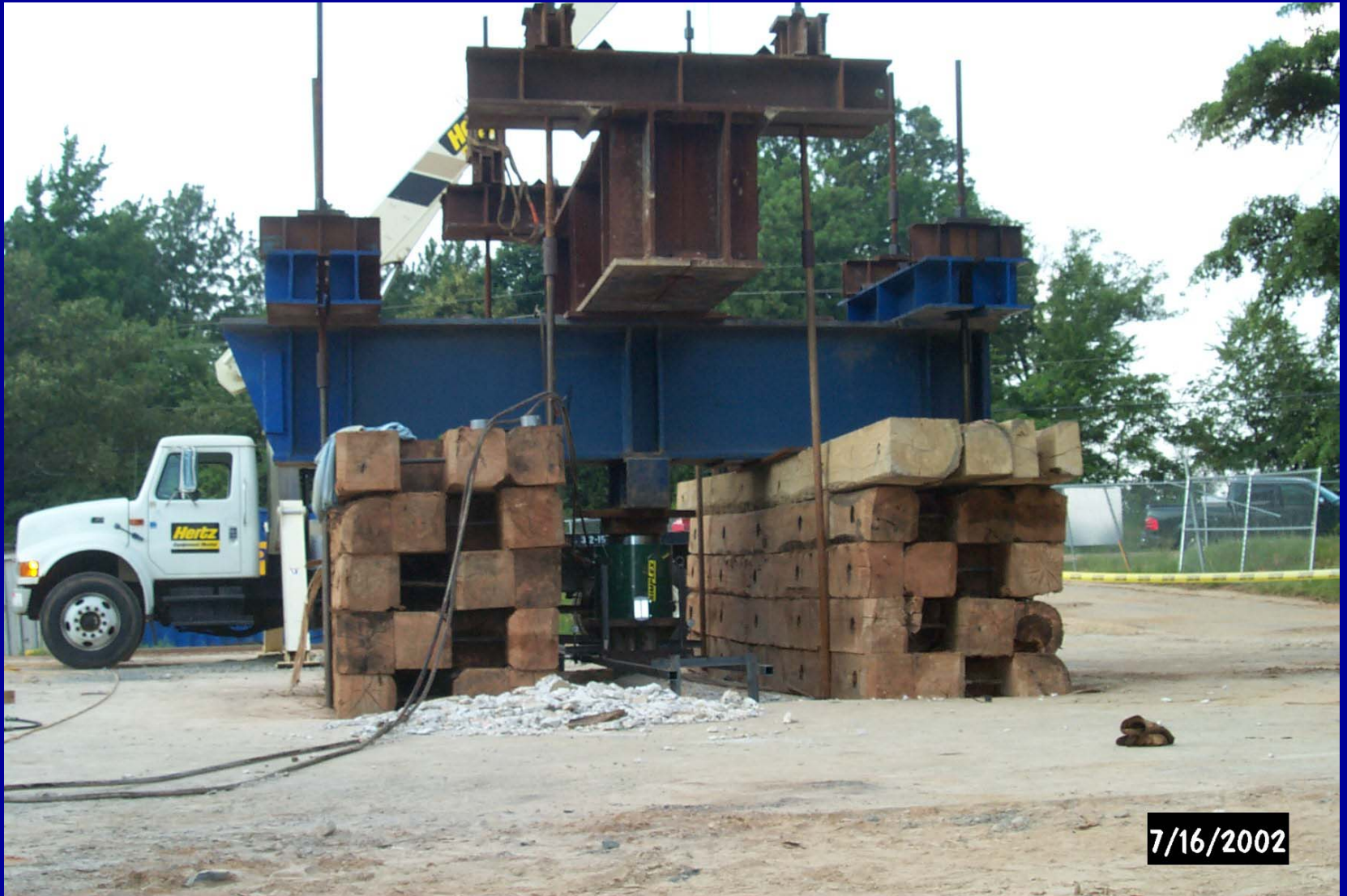
Double Reaction Beam Set-Up
