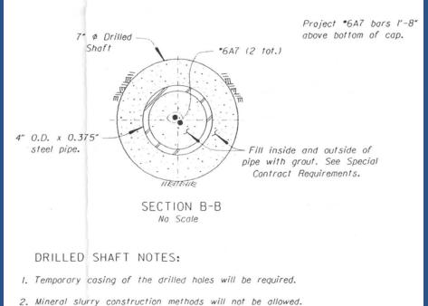
3. The bottom of the 4" O.D. x 0.375" steel pipe shall
